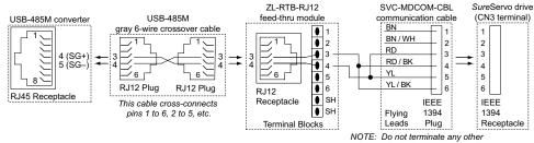
wires from this cable. Cut and tape them off. (The other wires are used by the SureServo drive.)
