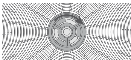
Fig.12 Hook the charcoal filter onto the locking clips and turn it clockwise.
