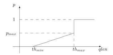
The queue length can be smoothed by specifying the wq parameter. The average queue length used in the tests are computed by the formula:
