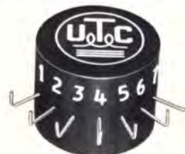
Instrument reference transformer. To operate from 15 kHz to 20 kHz with 12.5 V on one half of primary and to deliver 9.0 V on each half of secondary; secondary halves loaded with different im- pedances. Size: 1.1 Dia. max. x .79" high max. Weight: 34 gms.
