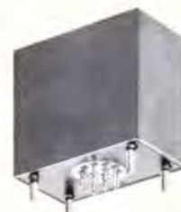
Bolometer transformer. Primary 10 ohms, secondary 530K ohms, 230:1 ratio, response from 1/2 Hz to 25 Hz. 120 db magnetic shielding, to 25 Hz. 120 db magnetic shield- plus full electrostatic shielding.
