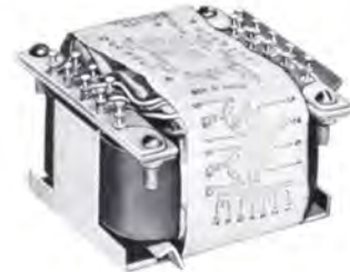
230° C. power transformer. Primary 115 V., 3 phase, 300/420 Hz to 200 V. and 20 V. secondaries, 525 V.A. 230° C. operating; 2¾ x 3 x 2", 1.8 lbs.
