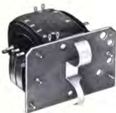
Scope power transformer with board for rectifiers. Primary 115 V., 400 Hz to two 14 KV filament windings, one 6.3 V. low capacity filament winding, 4.5 KV and 1.75 KV high voltage windings. 25 KV hipot when in oil; 2½ x 3½ x 2½", 1¼ lbs.
