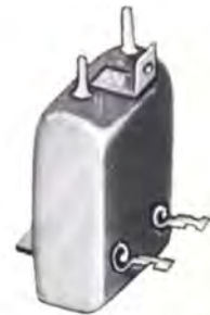
RF saturable inductor. 2 MA DC for sweep from 17 MHz to 21 MHz. MIL-T-27C; 2 oz.
