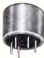
Molded carrier frequency trans- former, + 8 dbm level. Within 3 db from 100 Hz to 100 kHz. 4000:4000 ohms. 3/4 Dia. x 5/8 inches, 1/3 oz.
