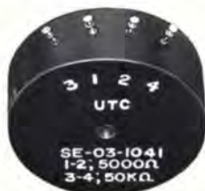
Toroidal transformer, primary 600 ohms, secondary 1200 ohms/split. From 1 kHz to 150 kHz, \pm 1 db at 10 mw max. Size: 1 1/8 Dia. x 3/8 inches. Weight: 25.6 grams. All types of toroidal transformers to specific requirements.
