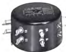
Toroidal Transistor inverter transformer. Input 24 V DC, outputs 4 windings 150 V to 1050 V DC. Hipot 3800 V. Hermetically sealed, MIL-T-27C, 2½ dia. x 1½, 15 oz.
