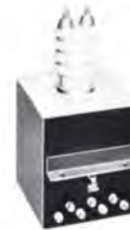
Low capacity current limiting filament transformer. Primary 118 V. 60 Hz to 6.3 V. at 3 A., 8 A. at short circuit. 25 MMFD capacity, 30 KV hipot and 200:1 capacity divider; 5 x 3¾ x 4½", 9 lbs.
