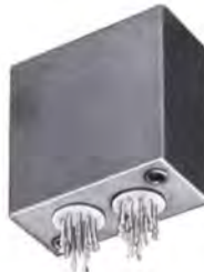
Precision reference transformer. Input 14 V., 400 Hz. Twelve secondaries held to low phase shift and .1% tolerance MIL-T-27C; 1¾ x 2 x 1¾, 4.5 oz.
