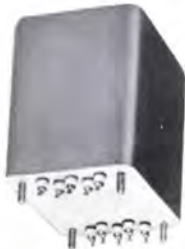
Magamp for 50 watt, 60 Hz servomotor. Two control windings. One feedback winding, one power winding, diode panel. Power gain 100. MIL-T-27C; 30 lbs.
