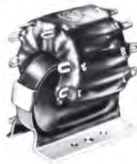
High temperature power transformer. Primary 115 V., 320/1000 Hz to four 6.3 V. and one 475 V. secondaries, 200° C. MIL-T-27C; 2¼ x 2 x 2", 9 ounce.
