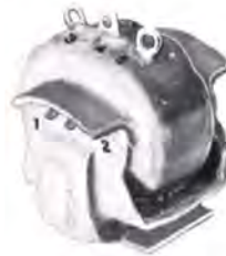
High voltage filament transformer. Primary 115 V., 380/1600 Hz to 5 VCT.-10 A., 21 KV hipot. 160° C. MIL-T-27C Grade 5; 2¼ x 2½ x 2¼", 10 ounce.
