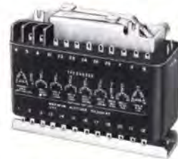
Molded Power Transformer 3 Phase. Input 200V, 380-420 Hz Electrostatic Shield, 8 output windings, 26 terminals. MIL-T-27C, Grade 2 Class S. Max. Alt. 50K Ft. Size 6 x 2½ x 5", 8 lbs.
