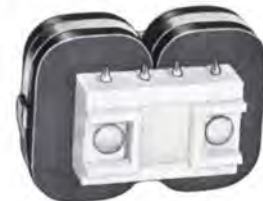
Molded High Temperature, High Voltage Transformer. Input 115 V 400 Hz, output 3400 V, 80 ma DC. Corona free molded terminals. MIL-T-27C Grade 5, Class T (170°C), 3¾ x 2¾ x 2½", 2 lbs. 10 oz.
