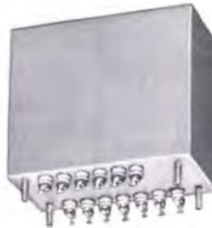
Servo reference transformer. Input 120 V., 380 to 420 Hz. Output ratios under load held to .005% tolerance. Phase shift .05° max. MIL-T-27C; 2¼ x 1¾ x 2, 12 oz.
