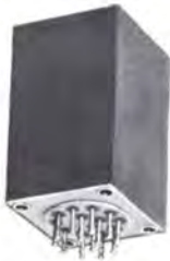
Two self saturating magamps in one case. Output 250 V. into 750 ohms. Power gain 135,000. MIL-T-27C; 2 x 2 x 2½, 12 oz.
