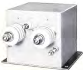
High Current and High Voltage Transformer. Input 115 V 400 Hz to 7.5 V CT-51A, 22 KV hipot. MIL-T-27C, Grade 4; 6½ x 6¾ x 6¾", 30 lbs.
