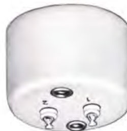
Constant 20 millihenries inductor. Inductance variation less than 2% from 0.1 to 500 V at 100 kHz. Q at 1 volt 100 kHz greater than 100. Case size: 1 1/8 O.D. x 1 3/16" high. MIL-T-27C.
