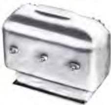
High temperature plate transformer. Primary 208 V., 3 phase 380/1000 Hz to 5100 V./leg, 1400 V. A. 200° C. MIL-T-27C; 6 x 3 x 4½", 6 lbs.
