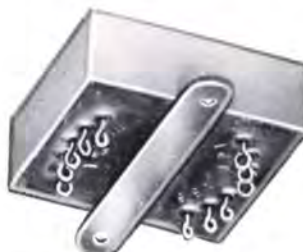
Instrument reference transformer. Input 50 V. 400 Hz. Three 5 V.-.025A. Outputs to .05% accuracy. Saturation characteristics and DCR balance to 3%. MIL-T-27C; 1½ x 1¾ x ¾, 2 oz.
