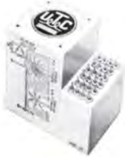
Power transformer; 3 phase input, one 12 phase and one 6 phase output. 25 VA total, MIL-T-27C, Class R. Size: 2 x 3 x 3".
