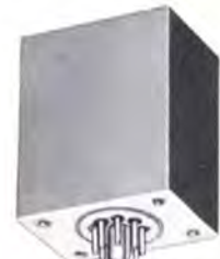
Magamp for 11 watt, 115 V., 400 Hz servomotor. Standard octal plug. MIL-T-27C; 1¾ x 2½ x 3, 1.7 lb.
