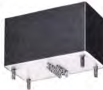
Precision Magnetic Modulator and Filter to produce sine wave output directly proportional to a DC control input. Temperature stabilized from -55°C to 85°C. Distortion and linearity less than 3% thru temperature and frequency range of 380-420 Hz. MIL-T-27C, 1½ x 1½ x 3½, 12 oz.
