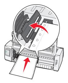
If necessary, move the left or right tractor to adjust the tractors to the paper width.
