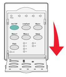
5 Press any paper movement button (Micro ↑, Micro ↓, or LineFeed) to move the paper to the Top-Of-Form position.
