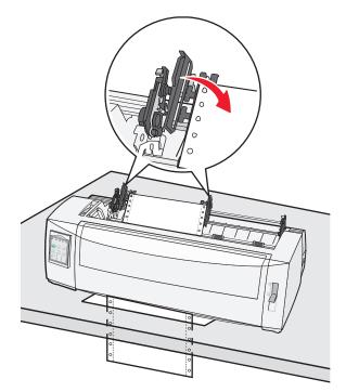
If necessary, move the left or right tractor to adjust the tractors to the paper width.
