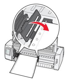
**9** Move the tractor to align the left margin on your paper with the **[A** symbol printed on the rear plate.
