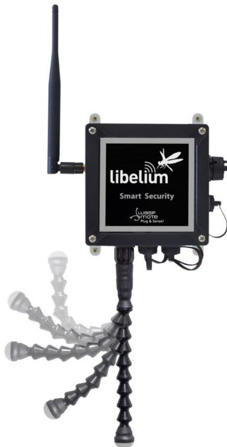
Figure: Image of configurations of the Presence sensor probe (PIR)
