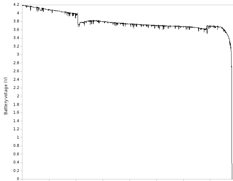
Figure: Typical discharging curve for battery
