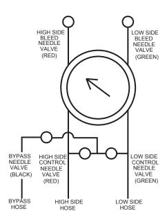
A "buffer" of less than 3 psi does not imply a leaking #1 check valve (i.e. allowing backflow) but rather is an indication of how well the #1 check valve is holding.
