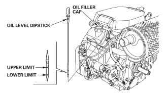
Oil is added to the engine by removing the oil cap and adding oil at this point. After filling the crankcase to the proper level, be sure you properly tighten the oil fill cap. NOTE: This engine generator must be on a level surface before you check or add oil to the system.
