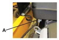
3. Engage the choke by pulling it out. A warm engine will require less choking than a cold engine.
