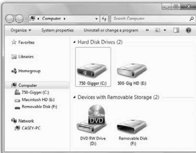
Figure 3-8: The Computer window is the starting point for any and all folder-digging. It shows the "top-level" folders: the disk drives of your PC. If you double-click the icon of a removable-disk drive (such as your CD or DVD drive), you receive only a "Please insert a disk" message, unless there's actually a disk in the drive.
