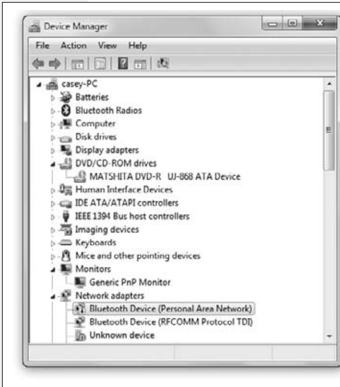
Figure 18-5: The Device Manager lists types of equipment; to see the actual model(s) in each category, you must expand each sublist by clicking the floppy triangle.
