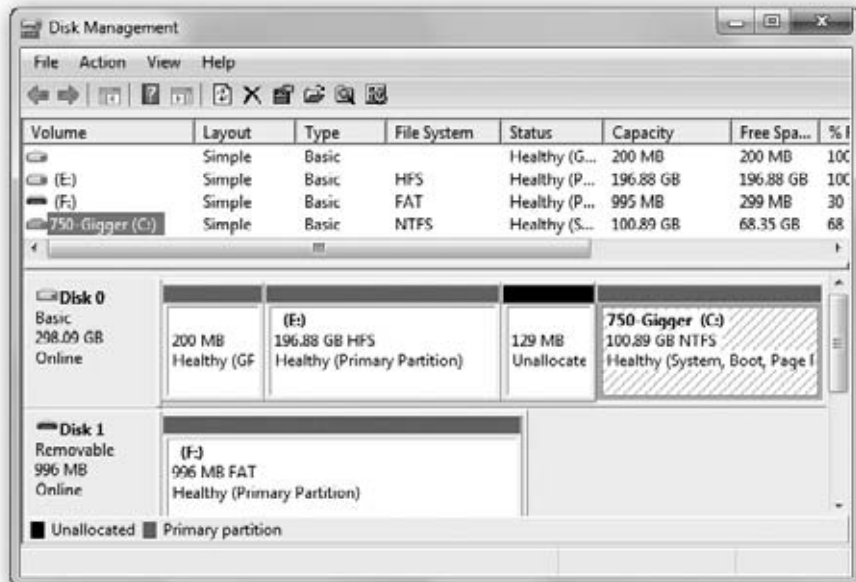
Figure 21-1: The Disk Management console is the central toolbox for all your disk-related tasks. This is where you create the dynamic volumes on your disks. Notice that drive E: is in trouble—it has no remaining free space. Read on for the solution.
