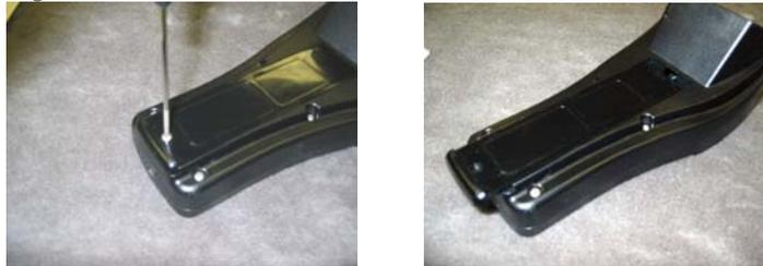
3. Remove the old cells from the compartment and replace them with fresh cells, following the orientation instructions on the inside of the access door.
