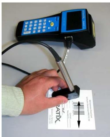
For best results, use a slower swipe speed for codes with narrower element sizes (such as < 100% Mag UPC, or Code 128), and faster swipes for less dense codes (such as Shipping Container codes). A good rule of thumb is to swipe as if you were underlining the code, or swiping a credit card at a retail checkout
