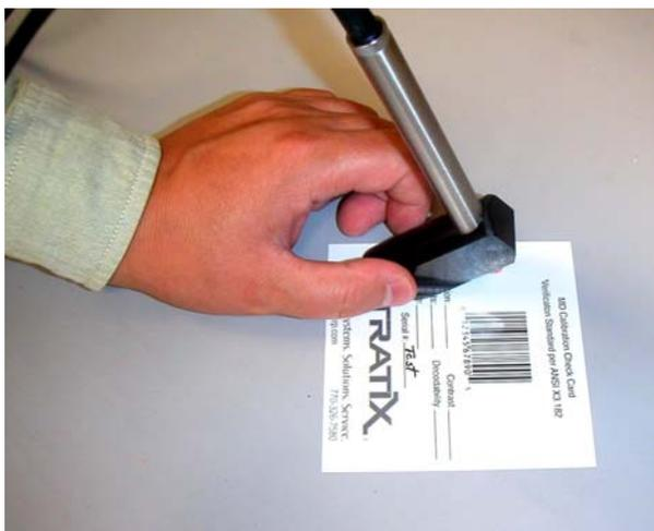
3. Begin with the wand tip outside of the bars in the code on either side of the code being tested. Grasp the sides of the wand guide with either hand to support the wand.
