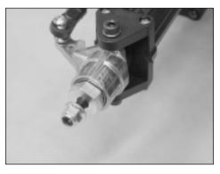
☐ Slide the new axle adapter into the steering knuckle, then reinstall the steering knuckle. Installation is the reverse of disassembly.
