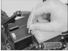
☐ Push the end of the antenna tube firmly into the molded hole in the top of the receiver box cover where the antenna exits.
