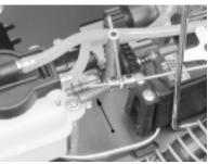
fails for any reason, the spring will manually pull the throttle closed, preventing a runaway truck.
