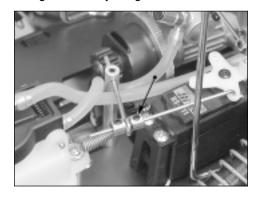
With the transmitter and receiver turned on, and the throttle/brake trim lever centered, the truck should roll smoothly (i.e., the brakes should be disengaged). If the brakes are dragging when the throttle trigger is at neutral, the brake discs will wear out very quickly. To ensure that the brakes are disengaged, always make sure that there is a 1/16" gap between the rear adjustment collar and the brake lever.
