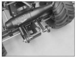
☐ Install the two wheelie bar assemblies onto the back of the chassis, using the drawing that comes with the wheelie bar set as a guide.
