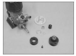
☐ The next step is to remove the stock clutch assembly from the engine. To do this, do the following: remove the steel hex screw from the end of the crankshaft, then remove the shims and pull the clutch bell off. Next, use a screwdriver to pry the large C-clip off of the crankshaft, then pull the clutch shoe assembly off. Lastly, remove the clutch nut and carefully pull the fly wheel and collet off of the crankshaft.
