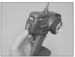
□ Slide the transmitter's on-off switch up to turn on the transmitter. The green LED should glow brightly.
