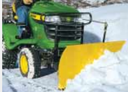
Front blade At 1.37 metres wide, it clears paths and drives with maximum ease.
