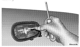
3. Pull the bulb straight from it's socket and replace.
