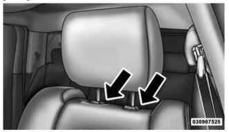
Removing Head Restraint
