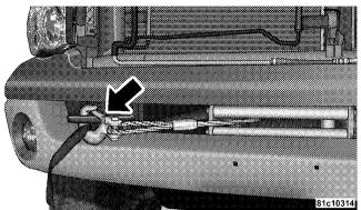
20. Disconnect the remote control. Disconnect the remote control cord from the control box and store in a clean and dry place. Winching operations are now complete. Put the cap on the solenoid plug-in.
