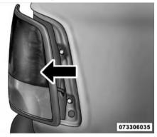
3. Disconnect the wiring harness connectors from the bulb socket.
