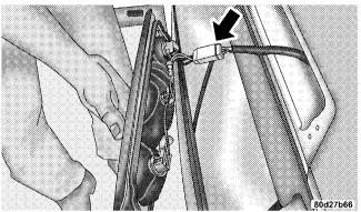
3. Turn the desired bulb socket 1/4 turn and remove the socket and bulb from housing.
