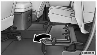
**Unfolding The Load Floor**
