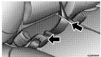
**Inserting Latch Plate**
