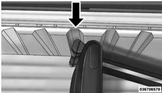
Aligning Gate To Slots
