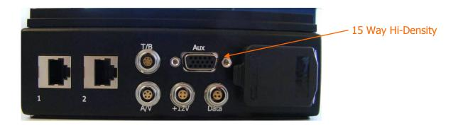
Take the 15-way High Density D-Type plug (Male) and connect it to the 15-way High Density D-Type jack (female) labelled AUX on the Phase 2 Plain Box NETNode.
