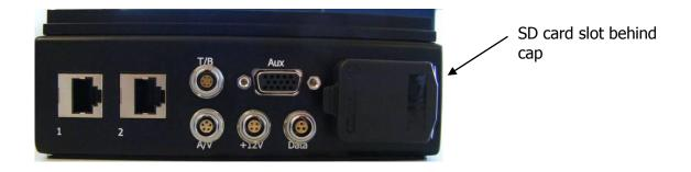
This will cause the green LED on the SD card slot to come on. The card should only be removed when the LED is green to prevent corruption of the data on the card.
