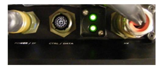
The LEDS are mounted behind a plastic 'flip' cover. The position and function is identical to the Phase 1 unit.
