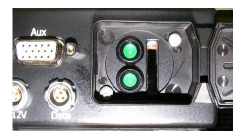
The LEDS are mounted behind a plastic 'flip' cover. The position and function is identical to the Phase  $\bf 1$  unit.
