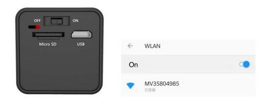
3. When the mobile phone is connected to the camera WiFi, open the mobile APP(V380 Pro) pull-down interface to refresh the data and automatically add the device
