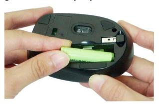
3. Replace the battery compartment cover back onto your mouse until it locks securely.
