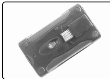
Snap receiver into the bottom of mouse
