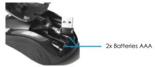
c) Take out the nano USB receiver and replace the cap.
