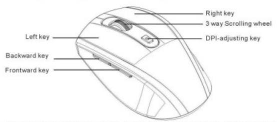
A)Using "DPI-adjusting key", the resolution of mouse can be switched between 800DPI and 1600DPI in turn. That LED light in "DPI-adjusting key" blinks slowly indicates 800DPI and fast 1600DPI.
