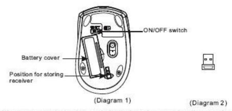
Whenever new batteries are installed, make sure that they are fresh 1.5V AAA batteries.
