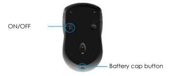
b) Insert two LR03 AAA 1.5V batteries (caution to the polarity).
