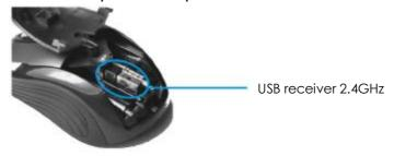
Switch on the mouse. Plug the nano receiver into your computer's USB port.
