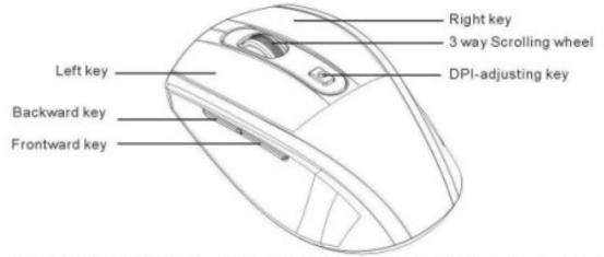
A)Using "DPI-adjusting key", the resolution of mouse can be switched between 800DPI and 1600DPI in turn. That LED light in "DPI-adjusting key" blinks slowly indicates 800DPI and fast 1600DPI.
