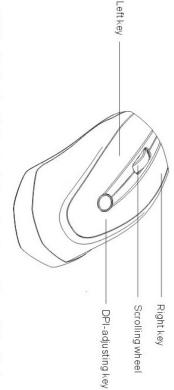
indicates 1000DPI and fast 1600DPI. 1000DPI and 1600DPI in turn. That LED light in "DPI-adjusting key" blinks slowly Using "DPI-adjusting key", the resolution of mouse can be switched between
