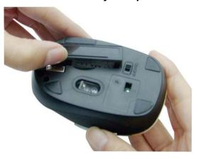
2. Install two AAA batteries into the battery compartment following the orientation guide in the battery bay.
