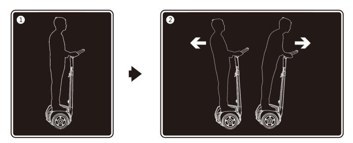
Step 4: Control the transverse direction of Robstep M2 When you swing the handle of Robstep M2 to the left, Robstep M2 turns left; when you swing the handle to the right, Robstep M2 turns right.
