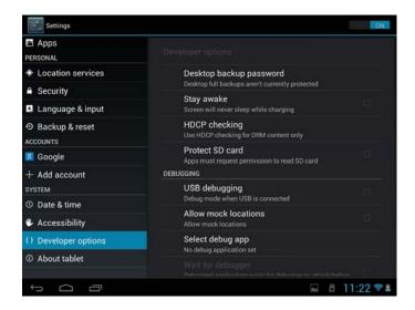
**USB debugging**: Check to permit debugging tools on a computer to communicate with your MR18 via a USB connection.
