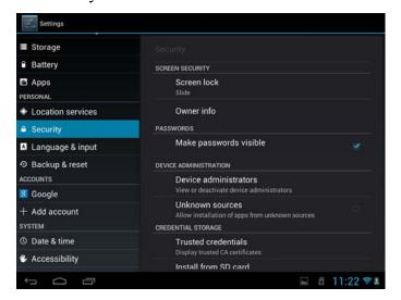
To set screen lock mode, tap **Settings** > **Security**> **Screen lock** to personalize the screen lock mode for you device.
