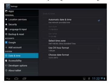
**Automatic:** Uncheck to set the date, time, and time zone on PE08 manually, rather than obtaining the current time from the mobile network.
