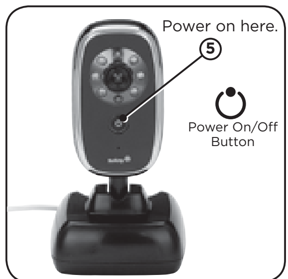
5 Turn Baby unit on. Hold down Power On/Off button until light comes on.
