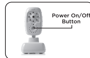
6 Hold down Power On/Off Button to turn Baby Unit on. To turn off Baby Unit, hold down Power On/Off Button again.
