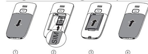
1. Remove the battery cover and the battery if it is already installed.
