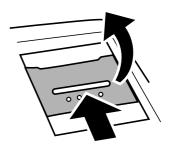
Lift the lid to an upright position. Place the card in the compartment. Make sure the contacts are facing downwards and the cut-off corner is placed as shown on the drawing. Hold the card in the correct position and close the lid.
