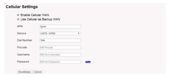
Note \*: For DLOS8 which doesn't have the cellular module, this page will shows Cellular not detected.
