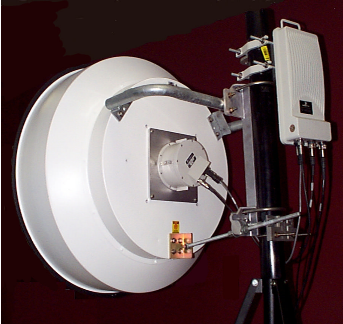
Figure 6-5 24 GHz system with 36" antenna mounted
