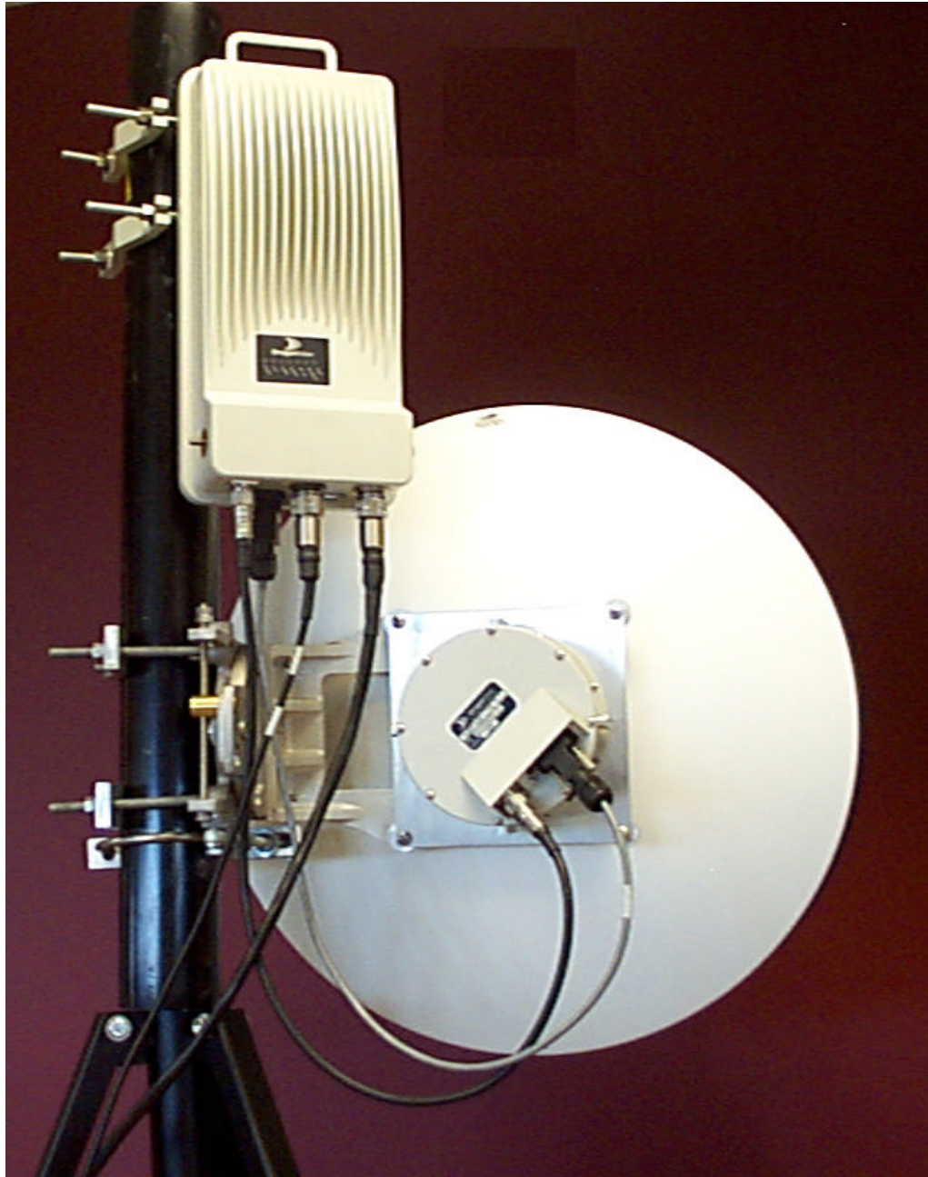
Figure 6-4 24 GHz system with 24" antenna mounted
