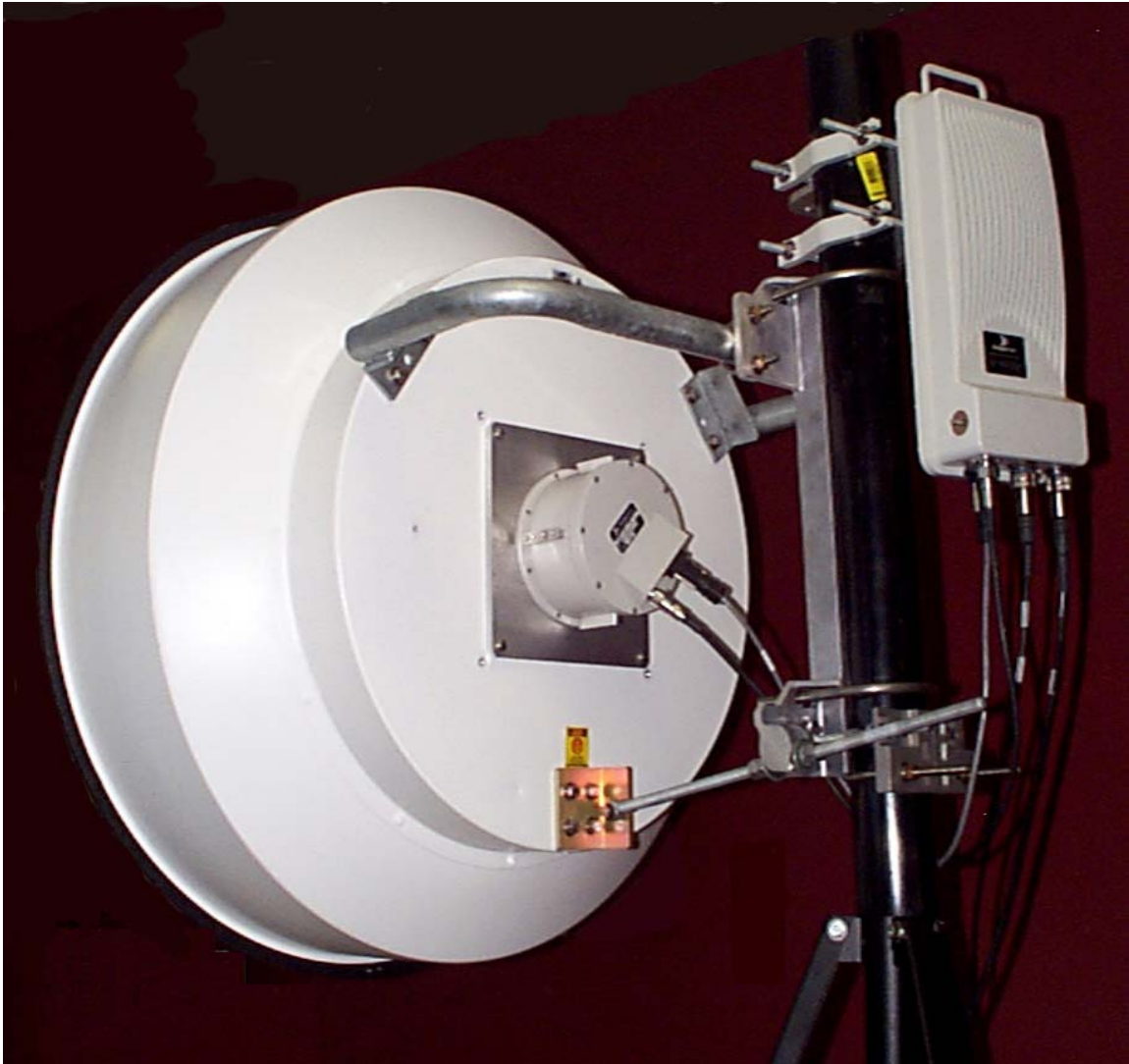
Figure 9 24 GHz system with 36" antenna mounted
