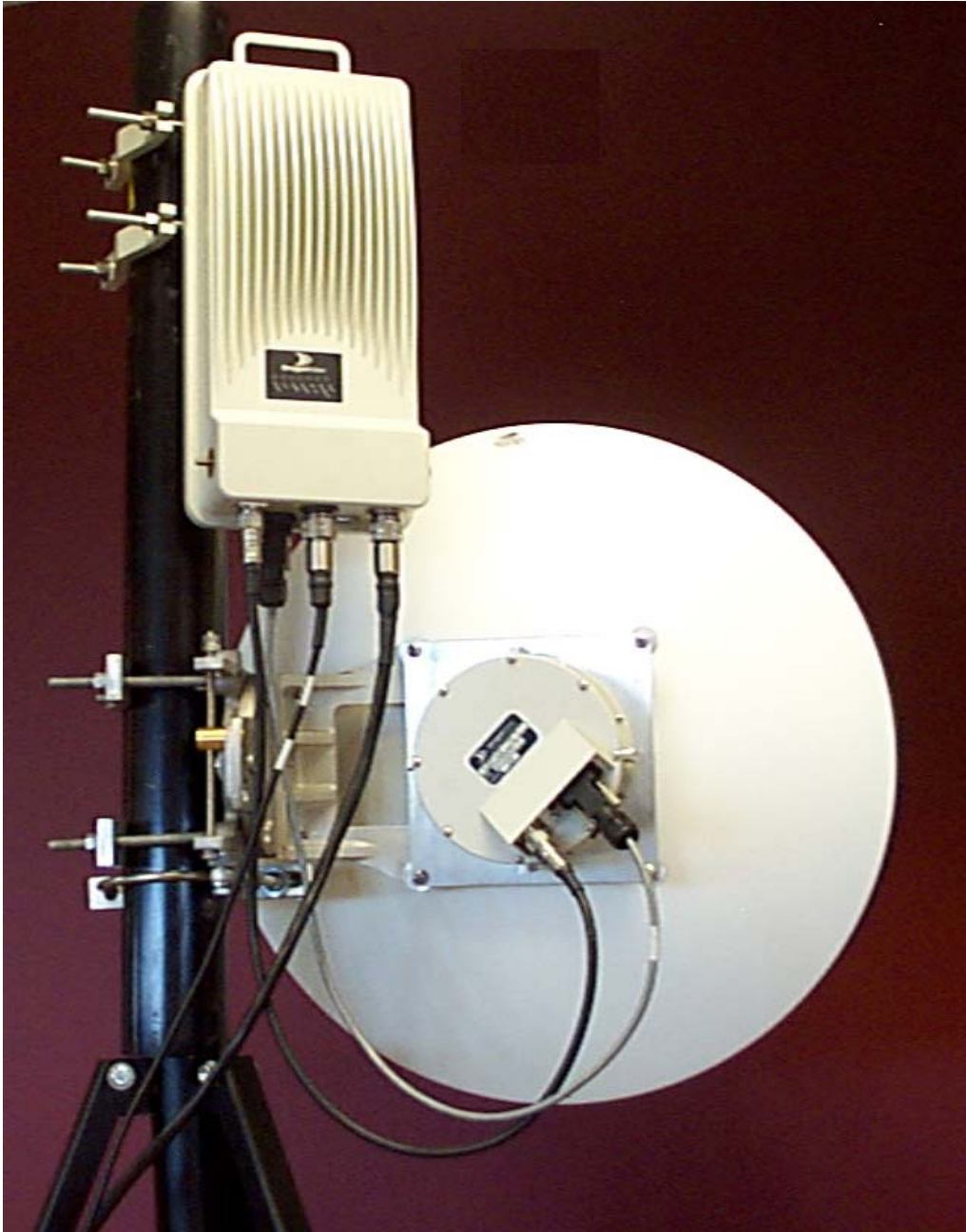
Figure 8 24 GHz system with 24" antenna mounted
