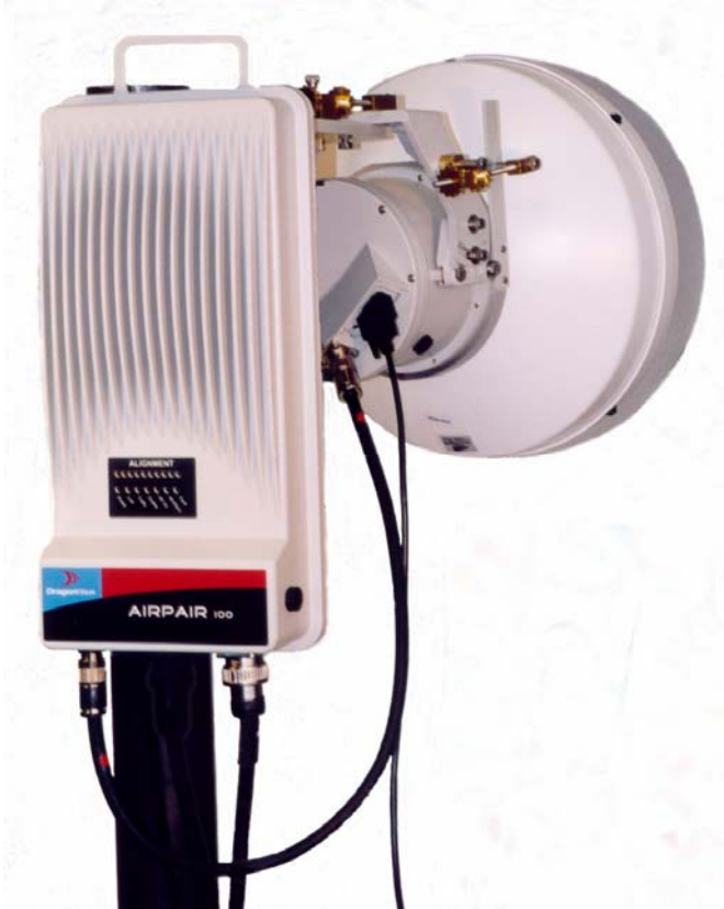
Figure 7 Alternative mount for 12" antennas
