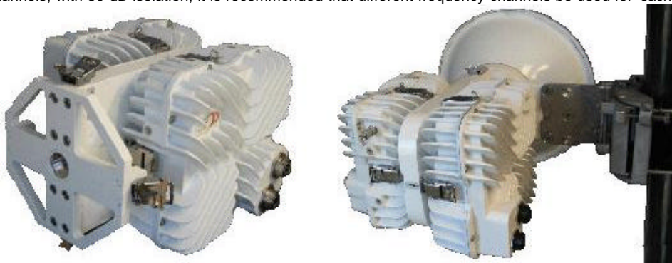
Figure 3-3 Dual Polarity Radio Mount
