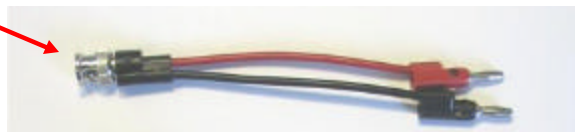
Figure 9-2 Voltmeter connections to BNC field strength monitoring connector
