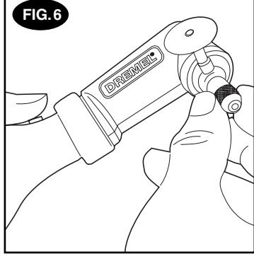
To change an accessory, insert the shank portion of any accessory (1/8" recommended) through the housing opening of the attachment to hold the shaft from rotating. With the shaft secured, loosen the collet nut and insert an accessory as deeply as possible to avoid wobble during use. (You may need to pull back the shank from the housing opening to provide clearance while inserting the accessory.) Retighten the collet nut.
