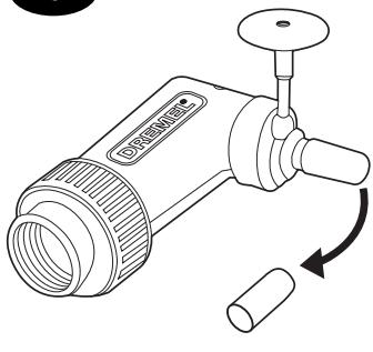
Before you begin, remove the black protective cap on your attachment. If cap does not slide off easily, insert the shank portion of any accessory (1/8" recommended) through the housing opening of the attachment to hold the shaft from rotating. Then twist off.
