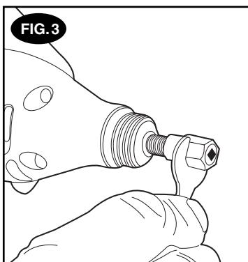
Install the drive adapter, included with your right angle attachment, on the motor shaft as shown in Fig. 3 and tighten.
