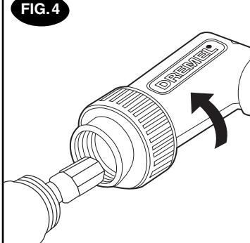
Screw the attachment onto your rotary tool. Hand tighten only. Reassemble the collet and the collet nut from step 2, on to the output shaft of the attachment.
