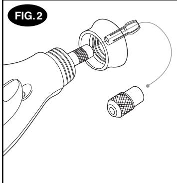
Remove the housing cap from your existing rotary tool as shown in fig. 2. Then press the shaft lock button on your rotary tool, unscrew the collet nut and remove the collet.
