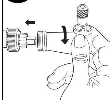
The Right Angle Attachment can be oriented on your rotary tool in 12 different positions. The attachment should be positioned so the on/off speed control switch is easy to access.
