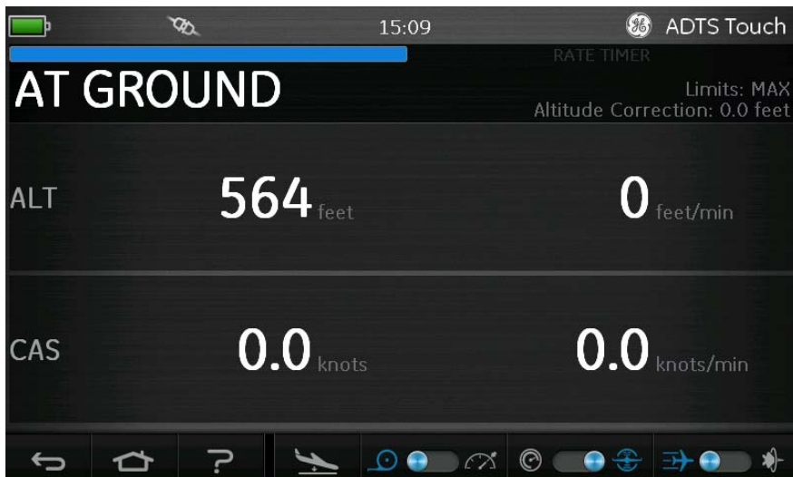
Figure 3-18 Go to ground complete
