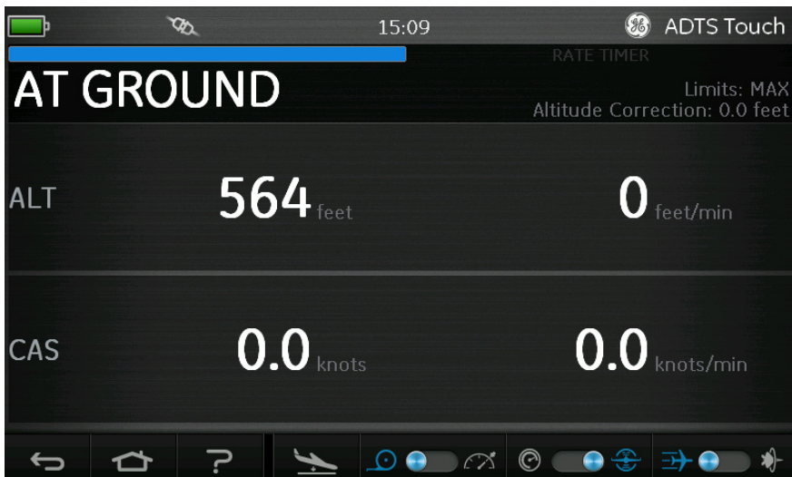
Figure 3-18 Go to ground complete
