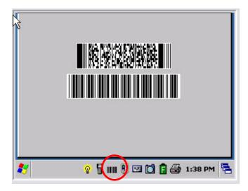
This is an emulation of the X3's barcode scanner. In an actual X3 handheld, touching the barcode icon or pressing the 'ACC' and 'B' keys will activate the barcode scanner. Aim the red laser to read 1D or 2D barcodes.
