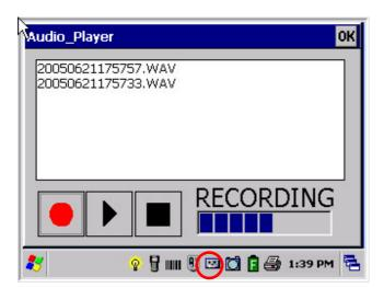
This is an emulation of the X3's audio applet. The audio applet can be launched by touching the icon in the system tray, or by pressing the 'ACC' and 'A' keys at the same time. The audio applet will automatically begin recording when launched. To stop recording and exit the applet, touch the square stop button. Recordings made during citation issuance will automatically be attached to the citation.
