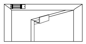
Single Lock, Inswing Door Mounted To Header Face With Adjustable Top Jam "Z" Bracket
