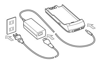
Connect the Cradle Connection Port (receptacle terminal) of the Unit into the USB Cradle, and then connect the AC Adapter to the USB Cradle.
