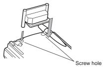
Fit the two protrusions of the Attachment Tool into the two screw holes of the Pocket PC to attach the Fixture to the Pocket PC.
