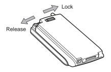
When you remove the Unit, slide the Lock Switch to the "Release" position before pulling out the Pocket PC.
