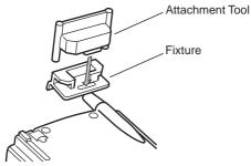
3 Peel off a protection seal of a double-faced tape on the back of the Fixture.
