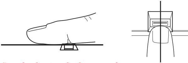
Sample aligning the finger on the sensor
