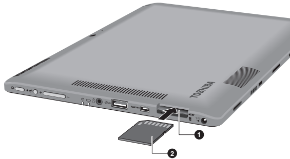
Figure 4-19 Inserting a memory media
