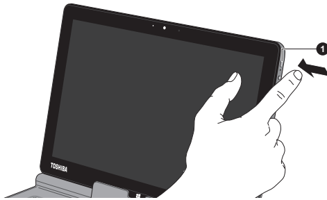
Figure 2-7 Turning on the power (laptop mode)
