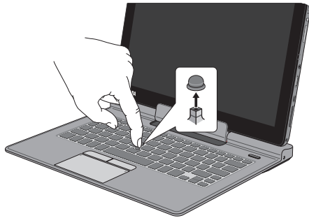
Figure 4-6 Removing the AccuPoint cap
