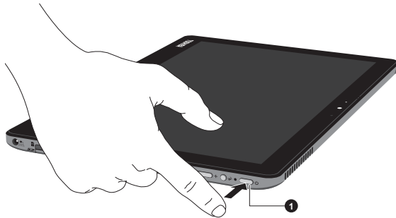
Figure 2-8 Turning on the power (tablet mode)
