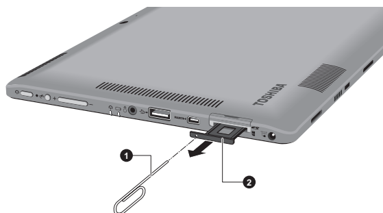
Figure 4-14 Open the SIM card tray
