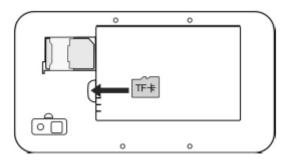
(2) Remove the memory card: Press down the MicroSD card, MicroSD card will automatically pop up and then remove the MicroSD card.
