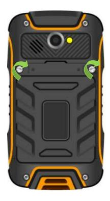
Turn the screw lock to the right on the battery cover till it locks.
