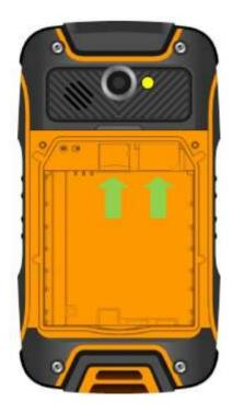
3. First match the lower part of the battery with the mobile phone metal part in the direction of Arrow 1 and then press the battery into the battery slot in the direction of Arrow 2.
