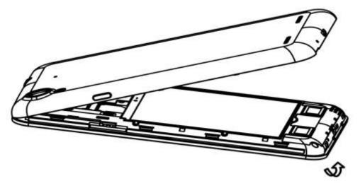
2, Take off the battery, put the SIM card into the corresponding card slot
