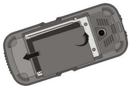
3. Replace the battery. Align the contacts of the battery with the corresponding connectors in the battery compartment.
