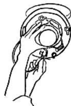
10 Remove the speaker grill by pushing one of the mounting clip screws towards the front of the speaker, then insert the speaker into the hole in the ceiling.
