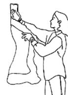
8 Pull the wires through the hole in the ceiling. Strip off the end of the outer wire jacket, then strip about  $\frac{1}{2}$  inch of the insulation from the ends of the wires.
