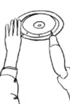
12 Reinstall the speaker grill by pushing it onto the speaker.
