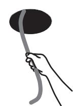
7 (Optional) To improve speaker performance, insert unbacked fiberglass insulation behind and around the speaker.
