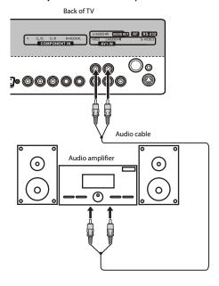
**Note:** Cable connectors and jacks are often color-coded. Match the colors when you connect the AV cable.
