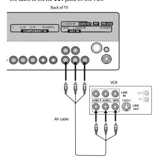
**Note:** Cable connectors and jacks are often color-coded. Match the colors when you connect the AV cable.
