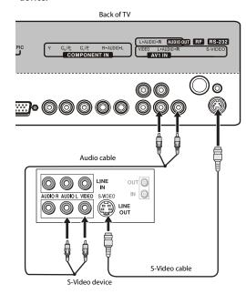
2 Connect one end of an audio cable (not included) to the AV1 IN L and R AUDIO jacks on the back of the TV, then connect the other end of the cable to the AUDIO OUT jacks on the S-Video device.
