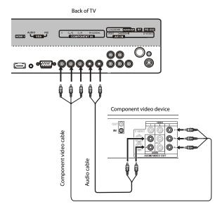
2 Connect one end of an audio cable (not included) to the L and R AUDIO jacks next to the COMPONENT IN video jacks on the back of the TV, then connect the other end of the cable to the L and R AUDIO OUT jacks on the component video device.
