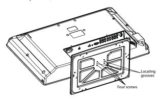
To remove the stand, loosen the four screws.
