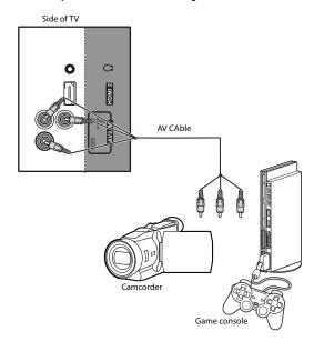
**Note:** Cable connectors and jacks are often color-coded. Match the colors when you connect the AV cable.
