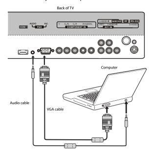
2 Connect one end of an audio cable (not included) to the VGA AUDIO jack on the back of the TV, then connect the other end of the cable to the AUDIO OUT jack on the computer.
