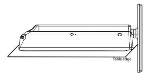
**6** Move the stand gently until the locators on the stand column align with the locating grooves on the stand, then use four screws (provided) to secure the stand to the column.
