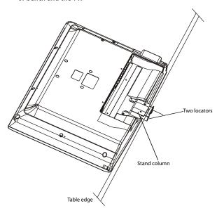
**3** Examine the stand carefully. The column socket is not in the center of the stand. You need to make sure you align the stand shown in the following illustration.
