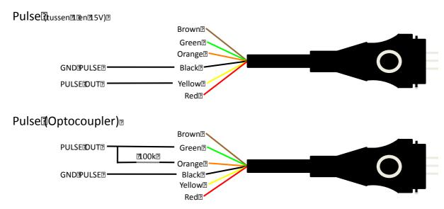
Note: A Optocoupler does not create any current-pulses. As the current pulses are measured by providing a current, a 110k resistor has to be installed between the orange and the green wire.
