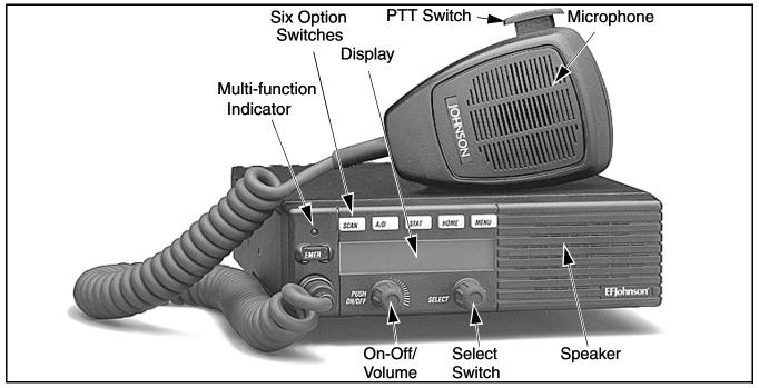
Figure 2-1 Front Panel Controls
