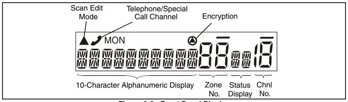
Figure 2-3 Front Panel Display
