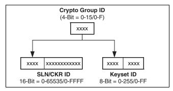
Figure 10-3 Encryption Parameter IDs
