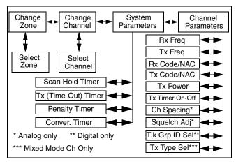
Figure 5-1 4300 Keypad Programming Menu Flowchart
