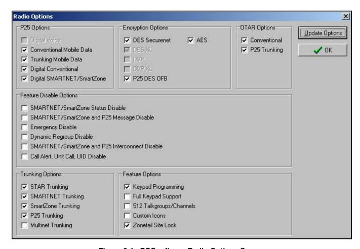
Figure 8-1 PCConfigure Radio Options Screen
