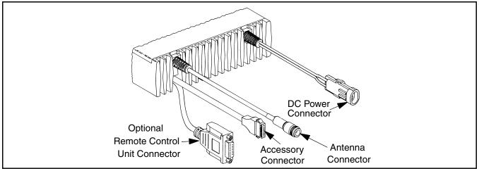
Figure 2-2 Rear Panel Connectors
